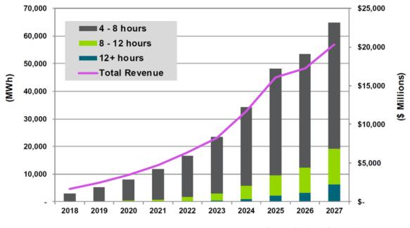
Annual Installed Long Duration Storage Energy Capacity and Deployment Revenue by Duration
